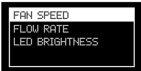
Fan speed: control the speed of the fan around the nozzle.
