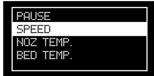
Speed: change the speed of the printhead while printing.
