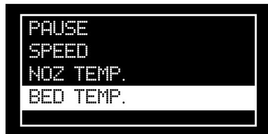
Buildplate Temp: change the buildplate temperature, especially useful for ABS printing.
