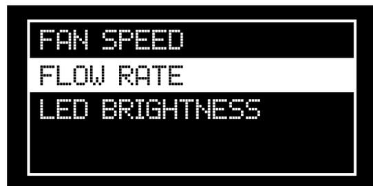
Material flow: control the amount of filament being supplied to the hotend nozzle.
