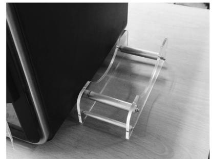
Place the filament spool on the right side of the printer.
