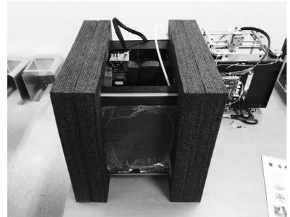
Remove the padded side rails from around the printer. Then grasp the bottom of the printer firmly and lift the printer out of the box.
