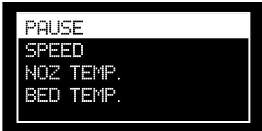
Pause: pause the machine while printing, commonly used to change filament.
