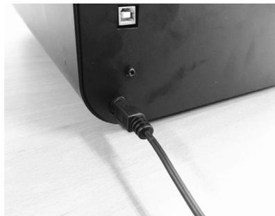
Connect the power adaptor to the rear of the printer and plug the printer in.
