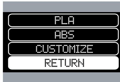
From the PLA/ABS/CUSTOMIZE/RETURN screen, turn the control dial to highlight the type of filament currently loaded in your printer and push in the control dial to start heating the hotend nozzle.
