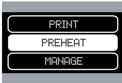
In main screen, turn the control dial to choose the preheat option. (picture) Push the control button in to select.
